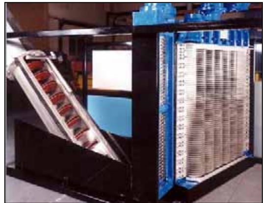
Screw Extraction Package Up to 13,900m 3 /h
